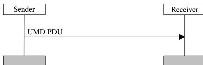
Figure 11.2: Unacknowledged mode data transfer procedure
