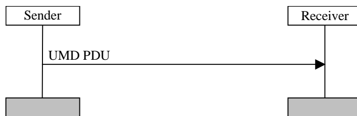
Figure 11.2: Unacknowledged mode data transfer procedure
