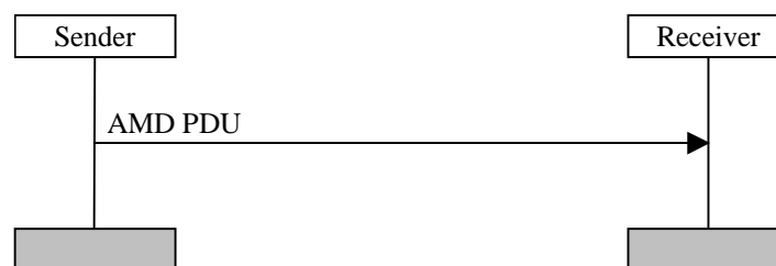
Figure 11.3: Acknowledged mode data transfer procedure
