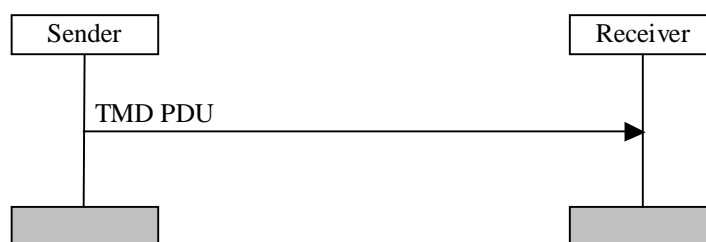
Figure 11.1: Transparent mode data transfer procedure
