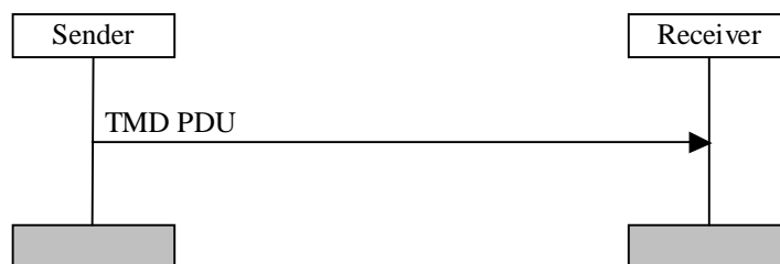
Figure 11.1: Transparent mode data transfer procedure
