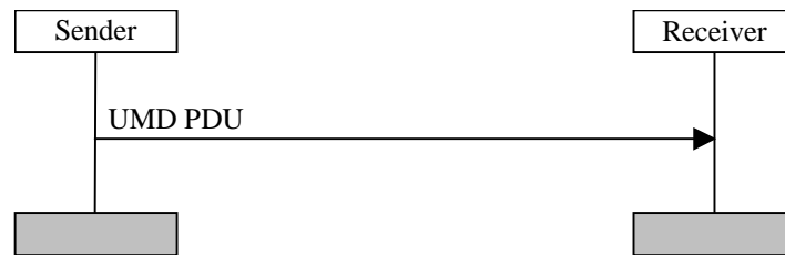
Figure 11.2: Unacknowledged mode data transfer procedure
