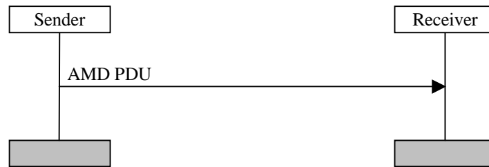
Figure 11.3: Acknowledged mode data transfer procedure
