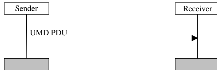
Figure 11.2: Unacknowledged mode data transfer procedure
