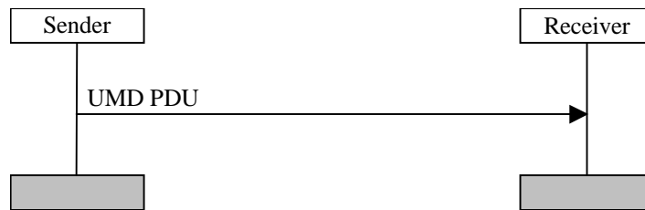
Figure 11.2: Unacknowledged mode data transfer procedure
