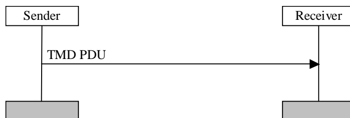
Figure 11.1: Transparent mode data transfer procedure
