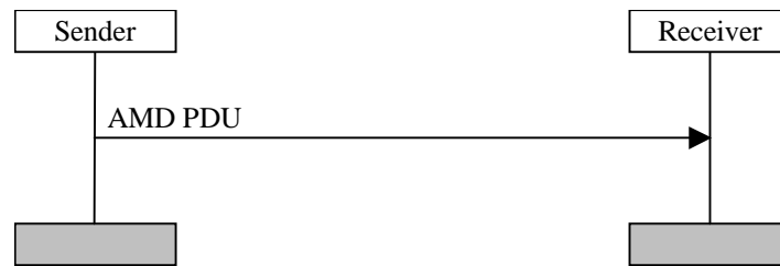
Figure 11.3: Acknowledged mode data transfer procedure
