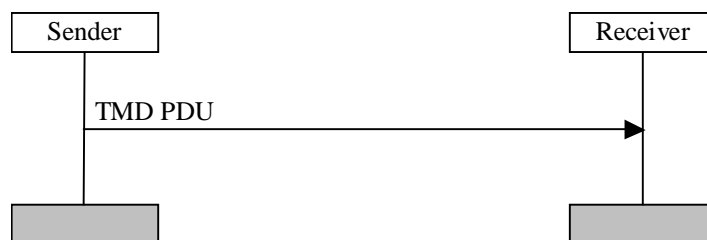
Figure 11.1: Transparent mode data transfer procedure
