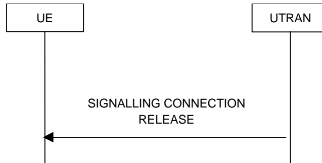
Figure 17: Signalling connection release procedure, normal case
