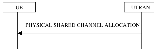
Figure 29: Physical Shared Channel Allocation
