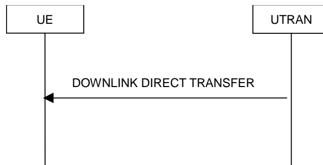
Figure 14a: Downlink Direct transfer, normal flow
