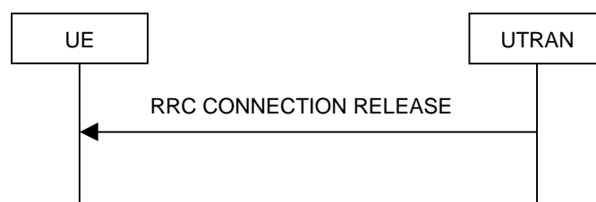
Figure 8.1.4-2: RRC Connection Release procedure on the CCCH
