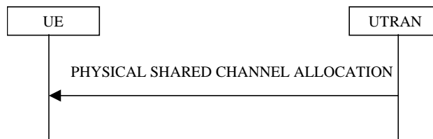
Figure 34: Physical Shared Channel Allocation
