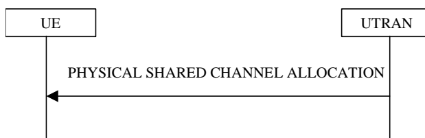
Figure 34: Physical Shared Channel Allocation
