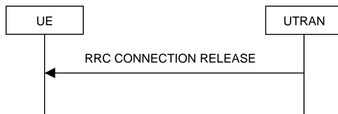
Figure 11: RRC Connection Release procedure on the CCCH
