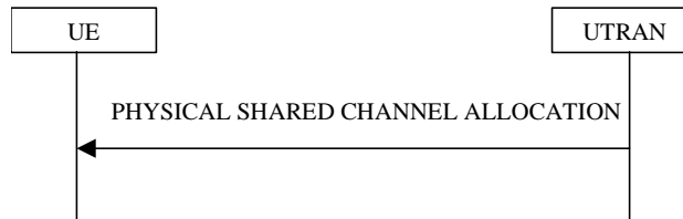
Figure 8.2.7-1: Physical Shared Channel Allocation
