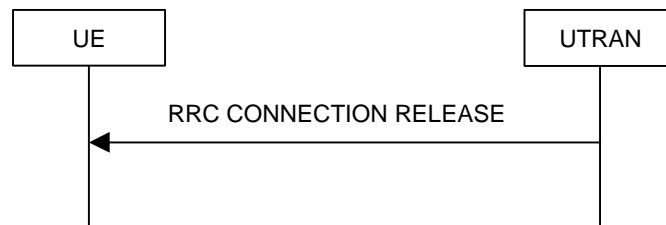
Figure 8.1.4-2: RRC Connection Release procedure on the CCCH
