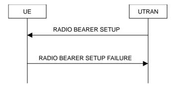
Figure 8.2.2-2: Radio Bearer Establishment, failure case
