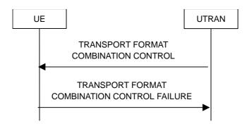
Figure 8.2.5-2: Transport format combination control, failure case
