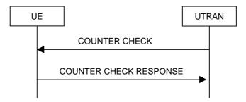
Figure 8.1.15-1: Counter check procedure
