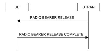
Figure 8.2.2-5: Radio Bearer Release, normal case
