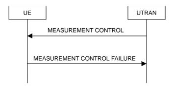
Figure 8.4.1-2: Measurement Control, failure case
