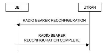
Figure 8.2.2-3: Radio bearer reconfiguration, normal flow
