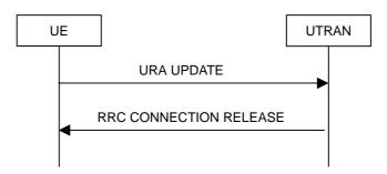
Figure 8.3.1-10: URA update procedure, failure case
