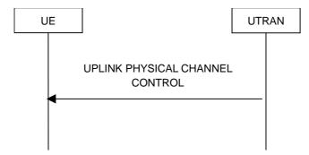
Figure 8.2.10-1: Uplink Physical Channel Control
