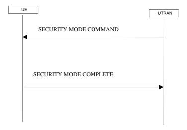
Figure 8.1.12-1: Security mode control procedure
