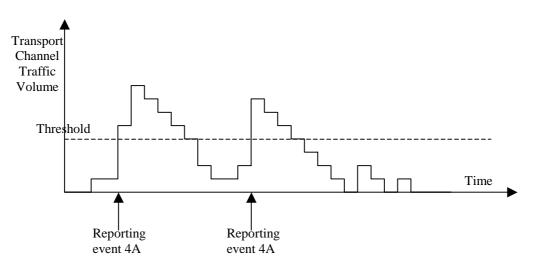
Figure 14.4.2.1-1: Event triggered report when Transport Channel Traffic Volume becomes larger than a certain threshold
