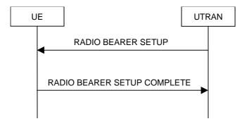
Figure 8.2.2-1: Radio Bearer Establishment, normal case
