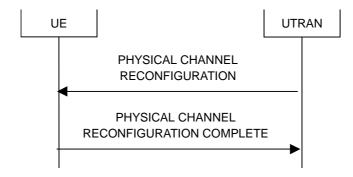
Figure 8.2.2-9: Physical channel reconfiguration, normal flow
