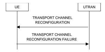
Figure 8.2.2-8: Transport channel reconfiguration, failure case
