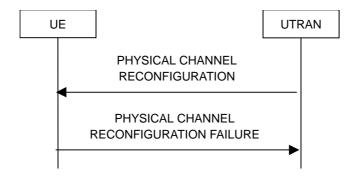
Figure 8.2.2-10: Physical channel reconfiguration, failure case
