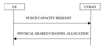
Figure 8.2.8-1: PUSCH Capacity request procedure
