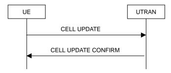
Figure 8.3.1-1: Cell update procedure, basic flow
