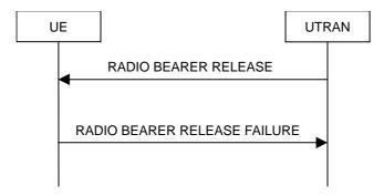
Figure 8.2.2-6: Radio Bearer Release, failure case
