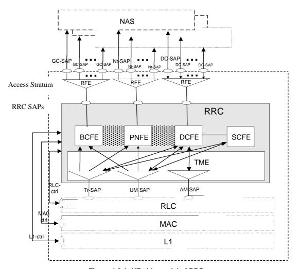
Figure 4.2-1: UE side model of RRC
