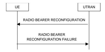
Figure 8.2.2-4: Radio bearer reconfiguration, failure case
