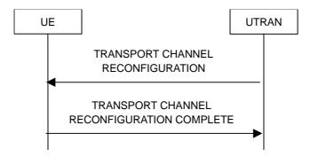
Figure 8.2.2-7: Transport channel reconfiguration, normal flow
