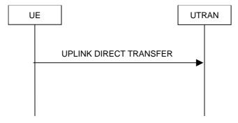
Figure 8.1.10-1: Uplink Direct transfer, normal flow
