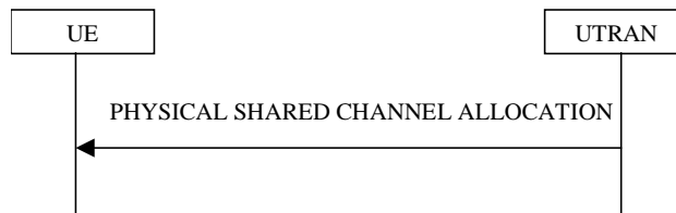
Figure 8.2.7-1: Physical Shared Channel Allocation
