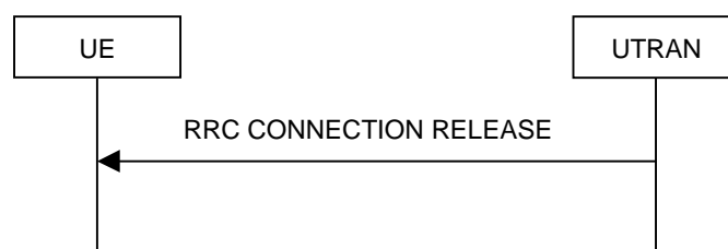
Figure 8.1.4-2: RRC Connection Release procedure on the CCCH
