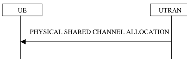
Figure 8.2.7-1: Physical Shared Channel Allocation
