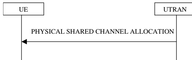
Figure 8.2.7-1: Physical Shared Channel Allocation
