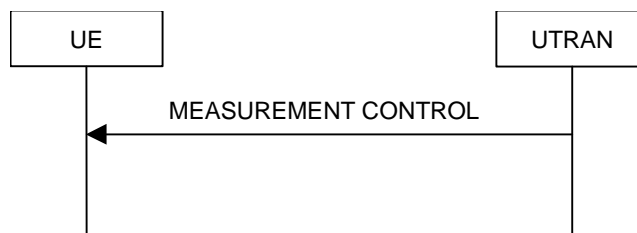
Figure 8.4.1-1: Measurement Control, normal case
