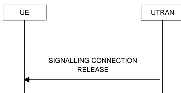
Figure 8.1.13-1: Signalling connection release procedure, normal case
