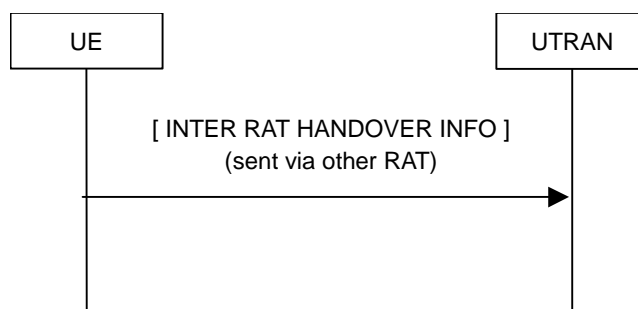
Figure 8.1.16-1: Inter RAT handover information transfer, normal flow
