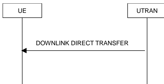
Figure 8.1.9-1: Downlink Direct transfer, normal flow
