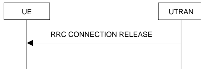
Figure 8.1.4-2: RRC Connection Release procedure on the CCCH
