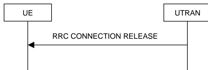
Figure 8.1.4-2: RRC Connection Release procedure on the CCCH
