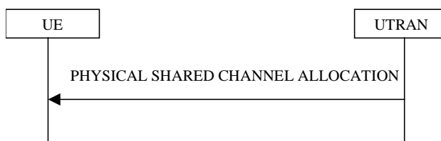
Figure 8.2.7-1: Physical Shared Channel Allocation
