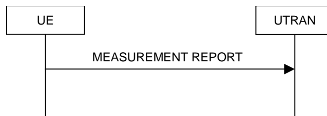
Figure 8.4.2-1: Measurement report, normal case
