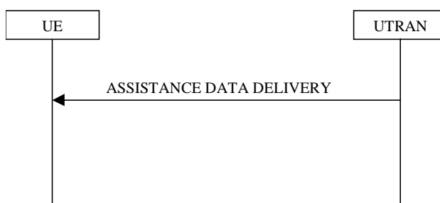
Figure 8.4.3-1 Assistance Data Delivery
