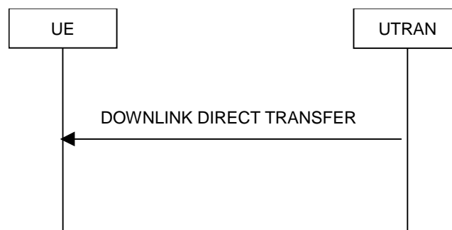
Figure 8.1.9-1: Downlink Direct transfer, normal flow
