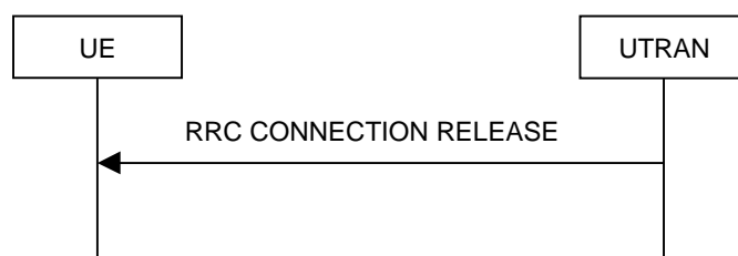
Figure 8.1.4-2: RRC Connection Release procedure on the CCCH
