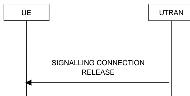
Figure 8.1.13-1: Signalling connection release procedure, normal case
