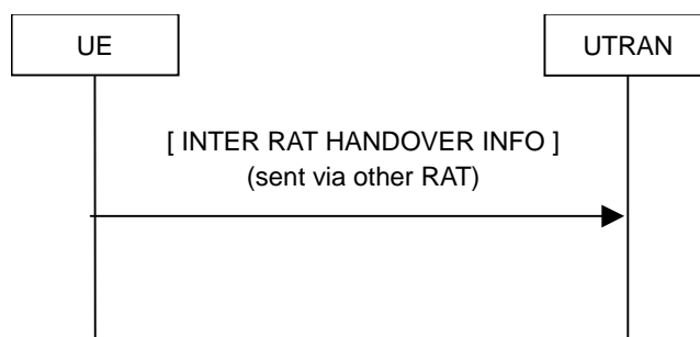
Figure 8.1.16-1: Inter RAT handover information transfer, normal flow
