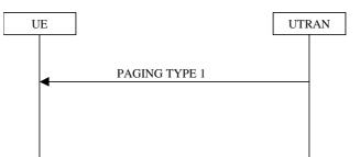
Figure 8.1.1-2: Notification of system information modification for UEs in idle mode, CELL\_PCH state and URA\_PCH state
