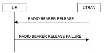
Figure 8.2.2-6: Radio Bearer Release, failure case
