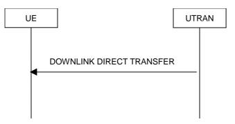
Figure 8.1.9-1: Downlink Direct transfer, normal flow
