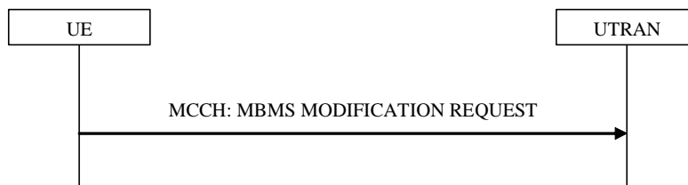
Figure 8.7.6-1: MBMS modification request, normal
