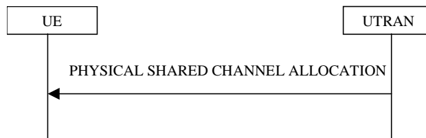
Figure 8.2.7-1: Physical Shared Channel Allocation
