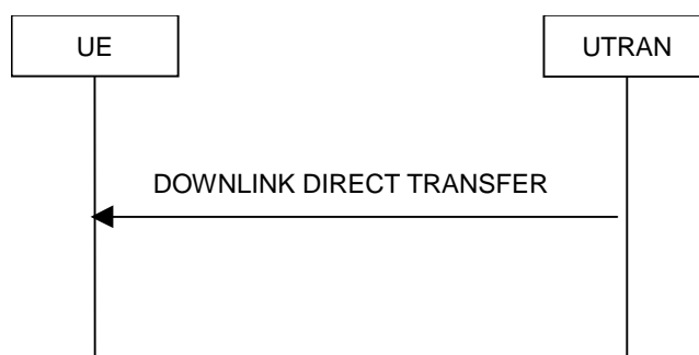
Figure 8.1.9-1: Downlink Direct transfer, normal flow
