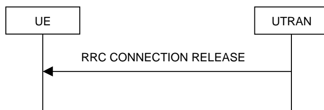
Figure 8.1.4-2: RRC Connection Release procedure on the CCCH
