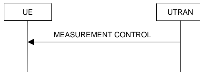
Figure 8.4.1-1: Measurement Control, normal case
