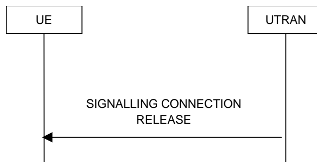
Figure 8.1.13-1: Signalling connection release procedure, normal case
