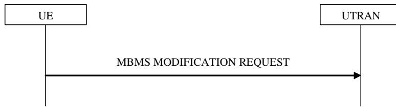
Figure 8.7.6-1: MBMS modification request, normal
