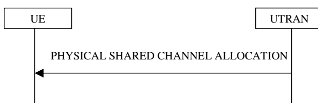
Figure 8.2.7-1: Physical Shared Channel Allocation
