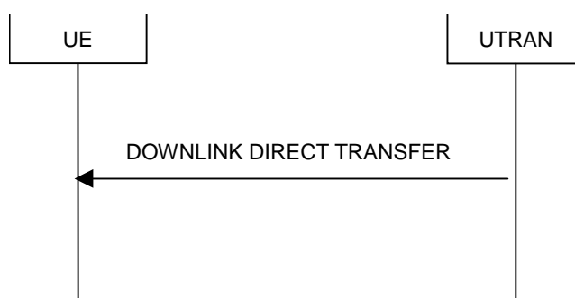
Figure 8.1.9-1: Downlink Direct transfer, normal flow
