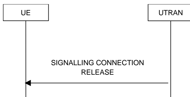
Figure 8.1.13-1: Signalling connection release procedure, normal case
