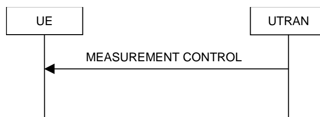
Figure 8.4.1-1: Measurement Control, normal case
