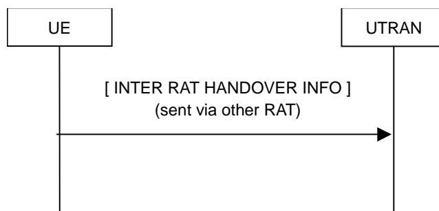
Figure 8.1.16-1: Inter RAT handover information transfer, normal flow
