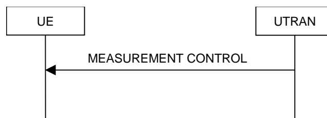
Figure 8.4.1-1: Measurement Control, normal case
