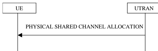
Figure 8.2.7-1: Physical Shared Channel Allocation
