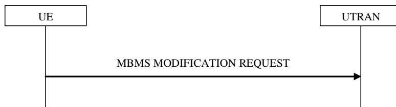
Figure 8.7.6-1: MBMS modification request, normal
