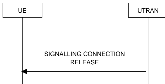
Figure 8.1.13-1: Signalling connection release procedure, normal case
