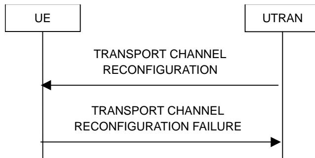
**Figure 8.2.2-8: Transport channel reconfiguration, failure case**
