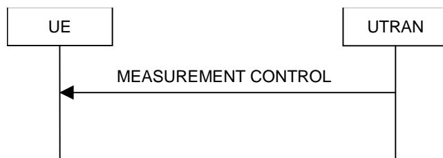
**Figure 8.4.1-1: Measurement Control, normal case**
