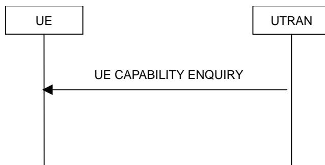
**Figure 8.1.7-1: UE capability enquiry procedure, normal flow**
