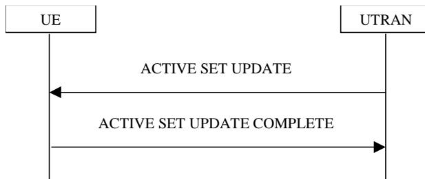
**Figure 8.3.4-1: Active Set Update procedure, successful case**
