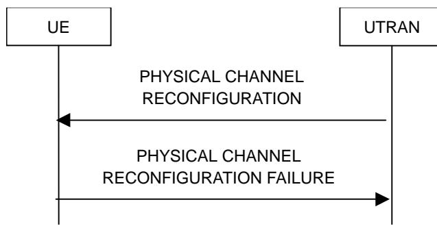
**Figure 8.2.2-10: Physical channel reconfiguration, failure case**
