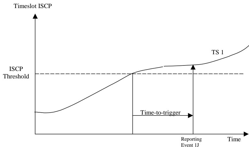
**Figure 14.1.5.2-2: Time-to-trigger limits the amount of measurement reports**
