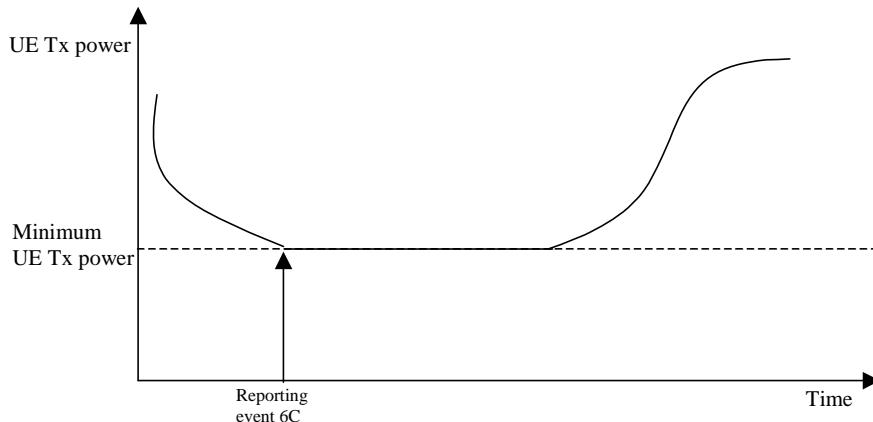
**Figure 14.6.2.3-1: Event-triggered measurement report when the UE Tx power reaches its minimum value**
