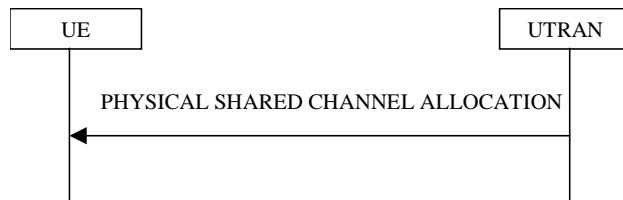
**Figure 8.2.7-1: Physical Shared Channel Allocation**
