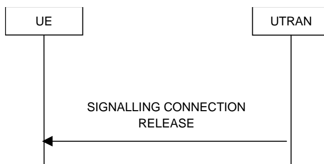
Figure 8.1.13-1: Signalling connection release procedure, normal case
