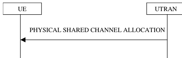
Figure 8.2.7-1: Physical Shared Channel Allocation
