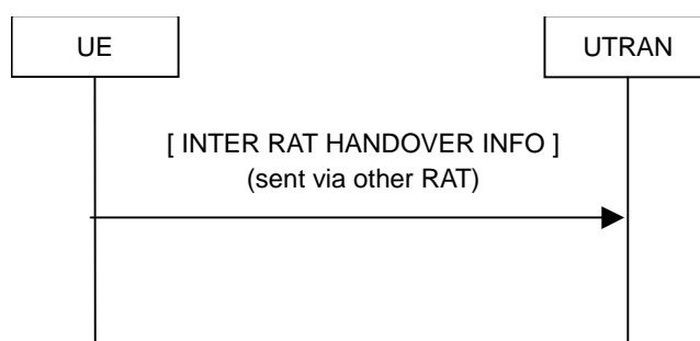
Figure 8.1.16-1: Inter RAT handover information transfer, normal flow
