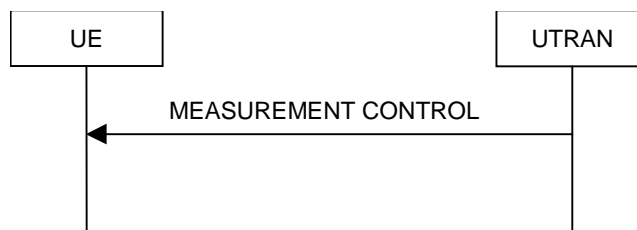
Figure 8.4.1-1: Measurement Control, normal case
