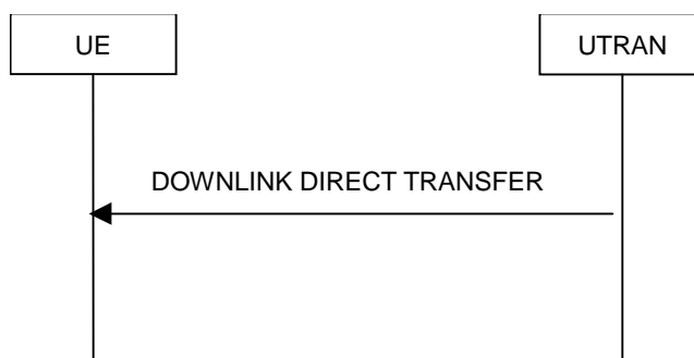
Figure 8.1.9-1: Downlink Direct transfer, normal flow
