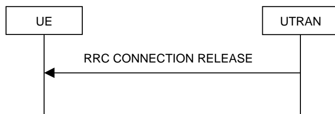
Figure 8.1.4-2: RRC Connection Release procedure on the CCCH
