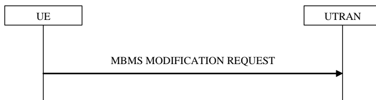
Figure 8.7.6-1: MBMS modification request, normal
