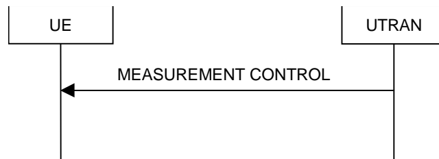
Figure 8.4.1-1: Measurement Control, normal case
