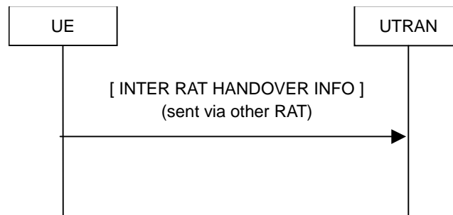
Figure 8.1.16-1: Inter RAT handover information transfer, normal flow
