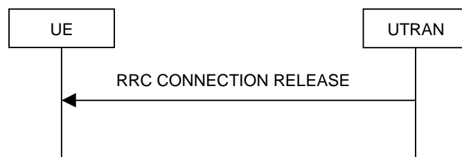
Figure 8.1.4-2: RRC Connection Release procedure on the CCCH
