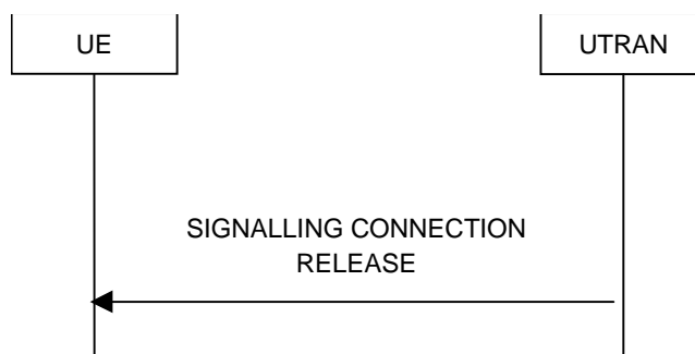
Figure 8.1.13-1: Signalling connection release procedure, normal case
