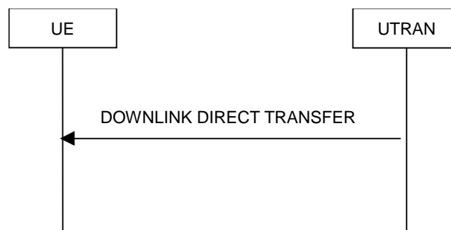
Figure 8.1.9-1: Downlink Direct transfer, normal flow
