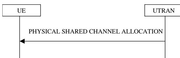
Figure 8.2.7-1: Physical Shared Channel Allocation
