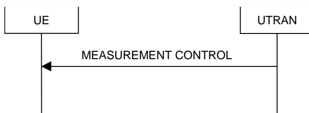
Figure 8.4.1-1: Measurement Control, normal case
