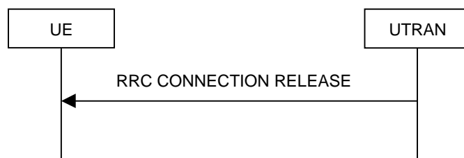
Figure 8.1.4-2: RRC Connection Release procedure on the CCCH
