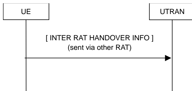
Figure 8.1.16-1: Inter RAT handover information transfer, normal flow
