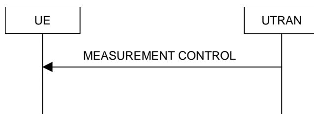
Figure 8.4.1-1: Measurement Control, normal case
