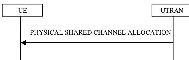
Figure 8.2.7-1: Physical Shared Channel Allocation
