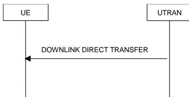
Figure 8.1.9-1: Downlink Direct transfer, normal flow
