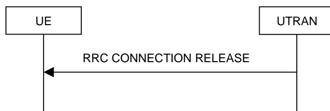
Figure 8.1.4-2: RRC Connection Release procedure on the CCCH
