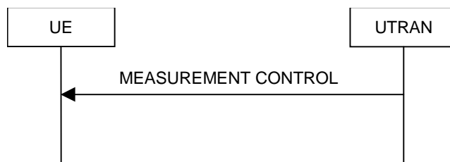
Figure 8.4.1-1: Measurement Control, normal case
