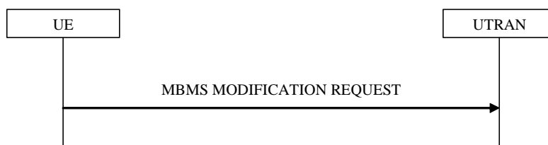
Figure 8.7.6-1: MBMS modification request, normal
