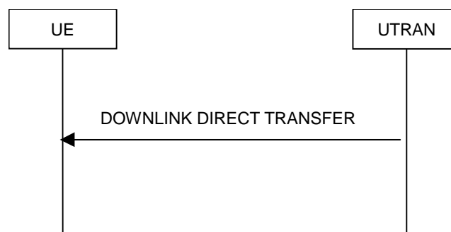
Figure 8.1.9-1: Downlink Direct transfer, normal flow
