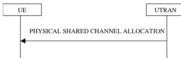
Figure 8.2.7-1: Physical Shared Channel Allocation
