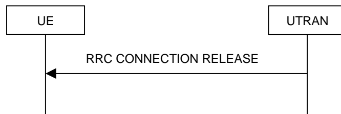
Figure 8.1.4-2: RRC Connection Release procedure on the CCCH
