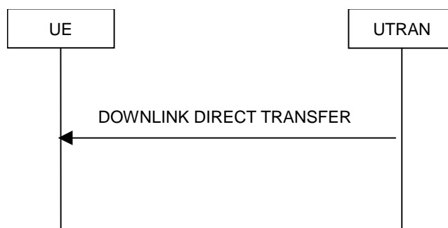
Figure 8.1.9-1: Downlink Direct transfer, normal flow
