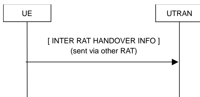
Figure 8.1.16-1: Inter RAT handover information transfer, normal flow
