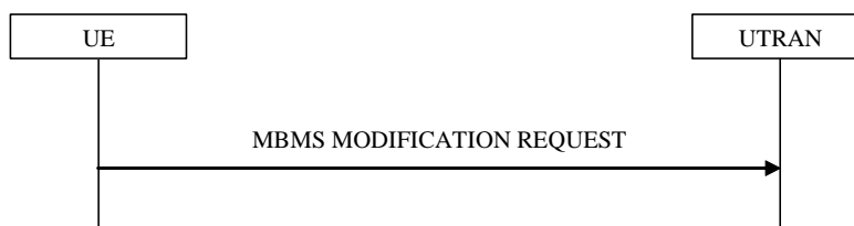
Figure 8.7.6-1: MBMS modification request, normal
