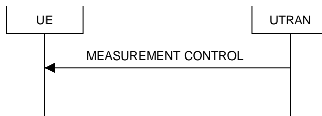
Figure 8.4.1-1: Measurement Control, normal case
