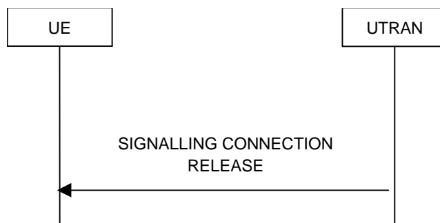
Figure 8.1.13-1: Signalling connection release procedure, normal case
