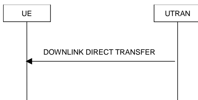
Figure 8.1.9-1: Downlink Direct transfer, normal flow
