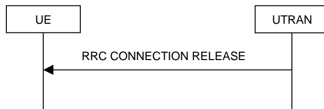
Figure 8.1.4-2: RRC Connection Release procedure on the CCCH
