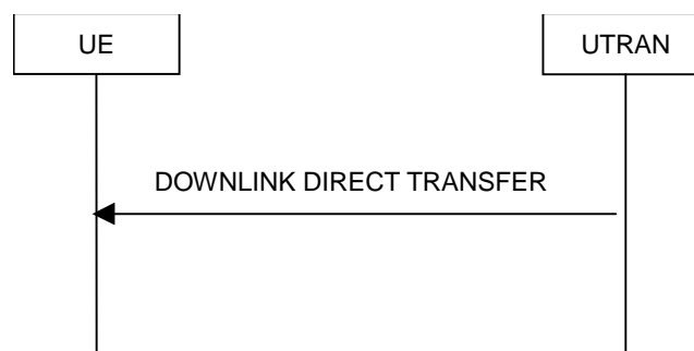
Figure 8.1.9-1: Downlink Direct transfer, normal flow
