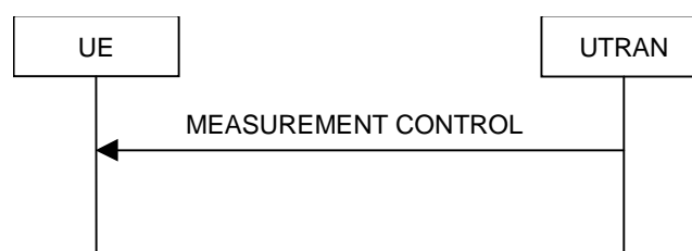
Figure 8.4.1-1: Measurement Control, normal case
