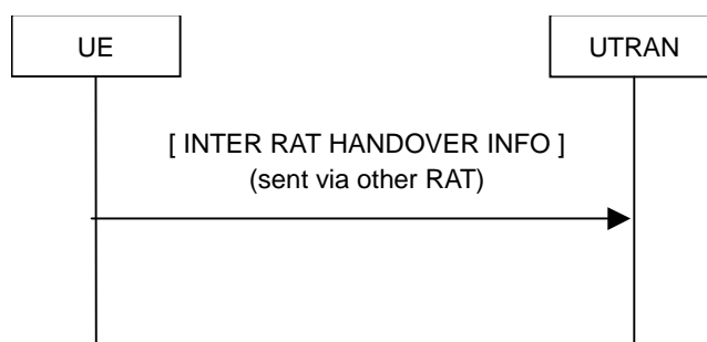
Figure 8.1.16-1: Inter RAT handover information transfer, normal flow
