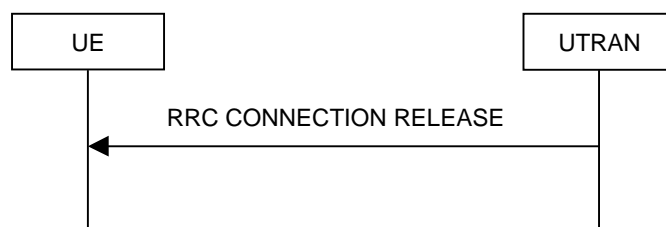
Figure 8.1.4-2: RRC Connection Release procedure on the CCCH
