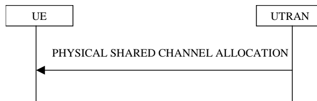
Figure 8.2.7-1: Physical Shared Channel Allocation
