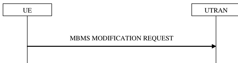
Figure 8.7.6-1: MBMS modification request, normal
