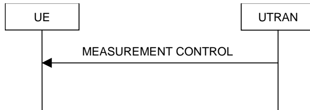
Figure 8.4.1-1: Measurement Control, normal case
