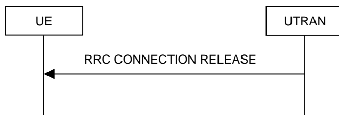
Figure 8.1.4-2: RRC Connection Release procedure on the CCCH
