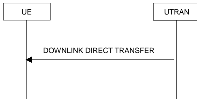
Figure 8.1.9-1: Downlink Direct transfer, normal flow
