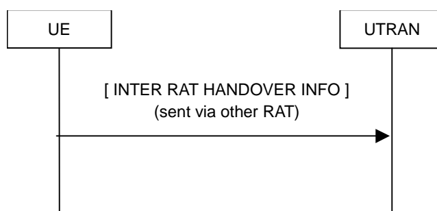
Figure 8.1.16-1: Inter RAT handover information transfer, normal flow
