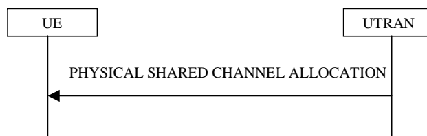
Figure 8.2.7-1: Physical Shared Channel Allocation
