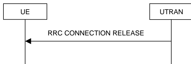
Figure 8.1.4-2: RRC Connection Release procedure on the CCCH
