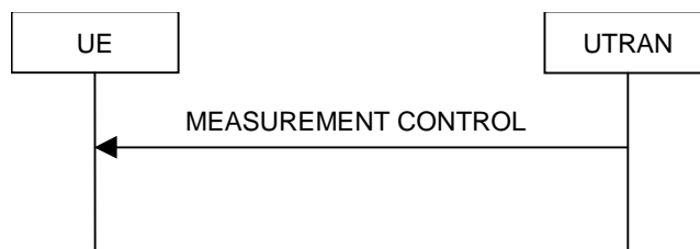
Figure 8.4.1-1: Measurement Control, normal case
