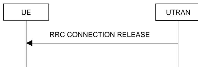
Figure 8.1.4-2: RRC Connection Release procedure on the CCCH
