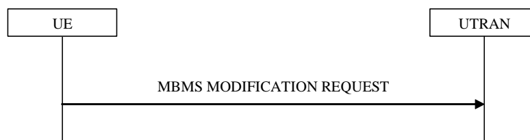
Figure 8.7.6-1: MBMS modification request, normal
