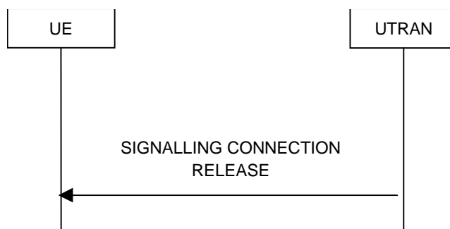
Figure 8.1.13-1: Signalling connection release procedure, normal case
