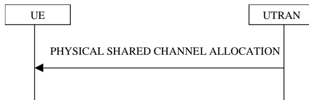
Figure 8.2.7-1: Physical Shared Channel Allocation
