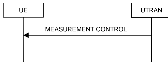
Figure 8.4.1-1: Measurement Control, normal case
