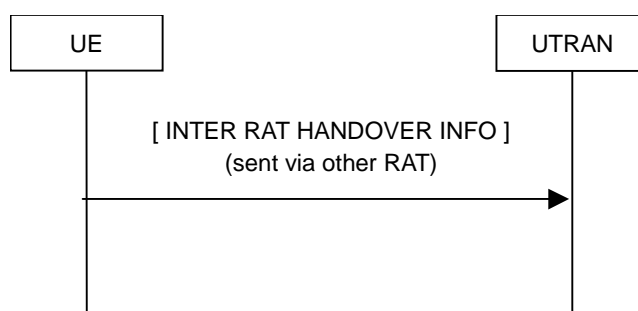
Figure 8.1.16-1: Inter RAT handover information transfer, normal flow
