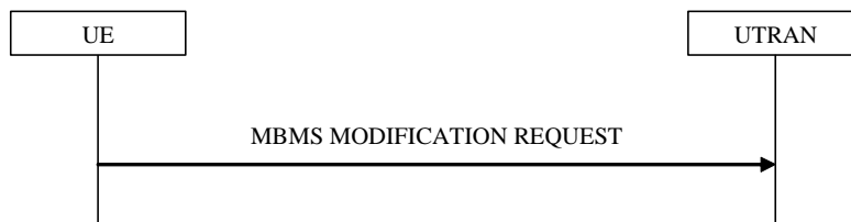
Figure 8.7.6-1: MBMS modification request, normal
