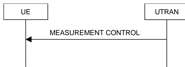
Figure 8.4.1-1: Measurement Control, normal case
