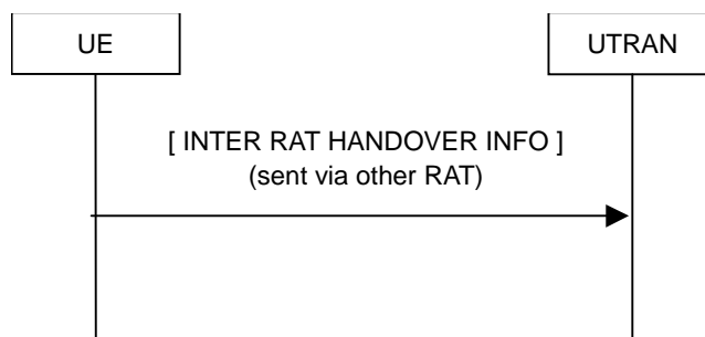
Figure 8.1.16-1: Inter RAT handover information transfer, normal flow
