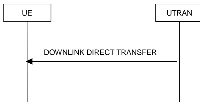
Figure 8.1.9-1: Downlink Direct transfer, normal flow
