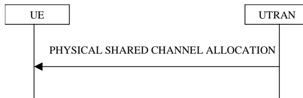
Figure 8.2.7-1: Physical Shared Channel Allocation
