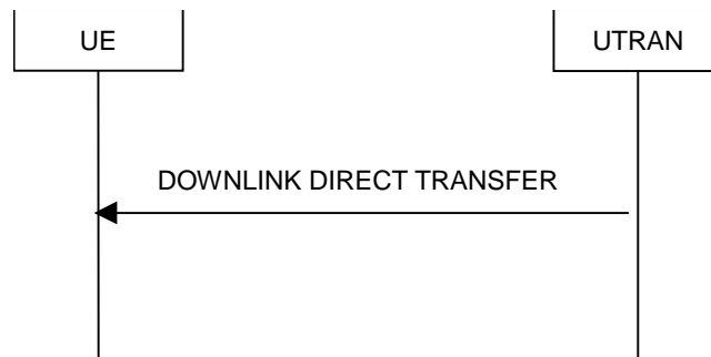
Figure 8.1.9-1: Downlink Direct transfer, normal flow
