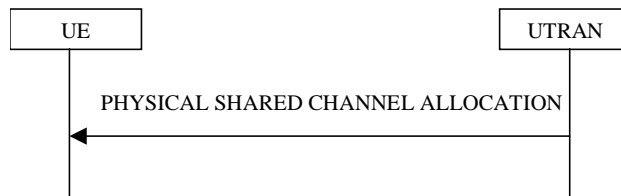
Figure 8.2.7-1: Physical Shared Channel Allocation
