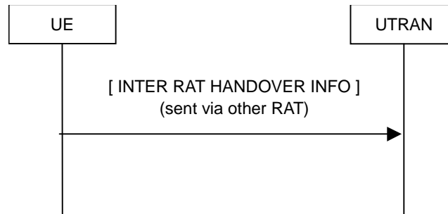
Figure 8.1.16-1: Inter RAT handover information transfer, normal flow
