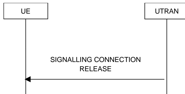
Figure 8.1.13-1: Signalling connection release procedure, normal case
