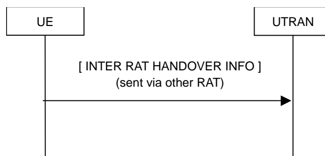
Figure 8.1.16-1: Inter RAT handover information transfer, normal flow
