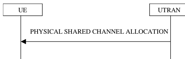
Figure 8.2.7-1: Physical Shared Channel Allocation
