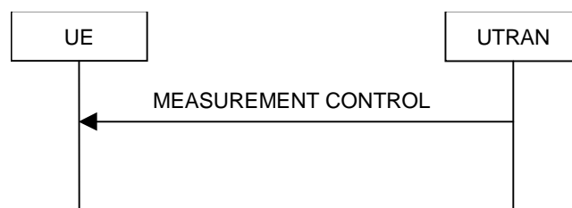
Figure 8.4.1-1: Measurement Control, normal case
