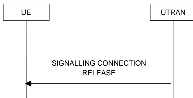
Figure 8.1.13-1: Signalling connection release procedure, normal case
