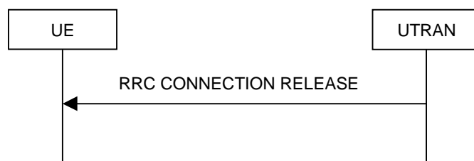
Figure 8.1.4-2: RRC Connection Release procedure on the CCCH
